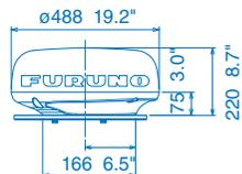
24" Radome Radar Sensor DRS4D-NXT 7.3kg 16.1 lb
